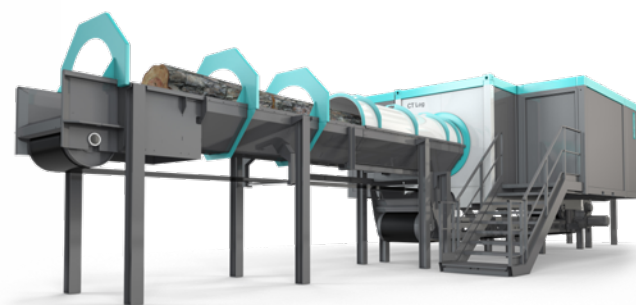
CT Log Computed Tomography for the sawmill of the future
